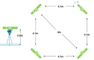
Fig. 2. Kinect arrangement setup. This setup was provided to ensure accurate data capture and synchronization.
