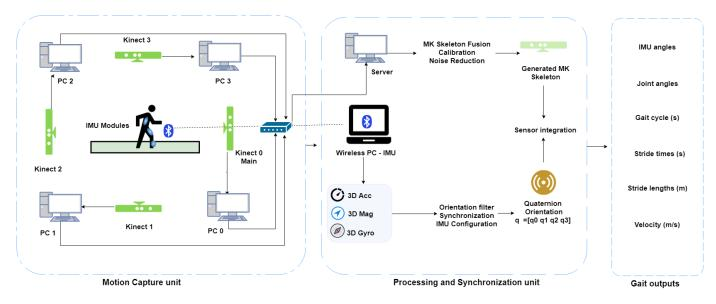
Fig. 1. Gait System diagram containing 4 Kinect skeletons and 4 IMU data as inputs and a fused 360° skeleton, angles, and gait spatiotemporal variables as outputs
