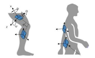
Fig. 5. IMU sensor placement and Euler rotation angle. Each IMU sensor has its own coordinate system and was calibrated before trials to ensure they are in the same coordinate system.
